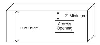
In order to use the minimum duct height, the door must be installed with it's longest dimension running horizontally along the length of the duct. If the minimum duct height is used, the top of the opening must be 2" from the top of the duct. For every inch over the minimum duct height, the opening can be lowered 1" from the top of the duct.
