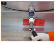
4. Insure the bucket hose clamp is in place and slide the bucket hose on the PVC fitting.
