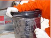
6. Remove the wrap from the container exposing 16 water drain holes.
