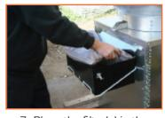
7. Place the filter(s) in the box. One filter for 4" and two filters for 7".
